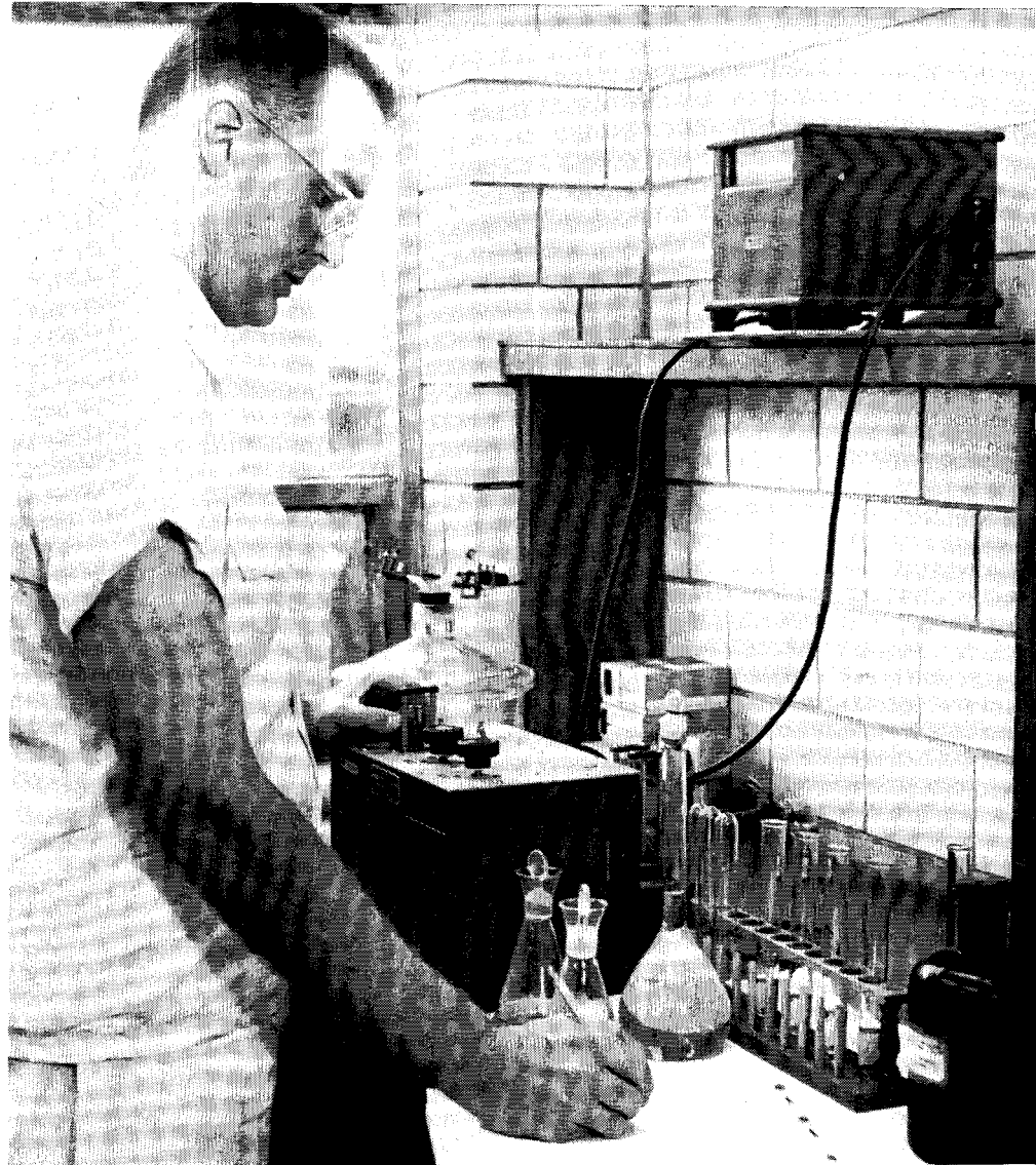
Vitamin determination with a photoelectric colorimeter
